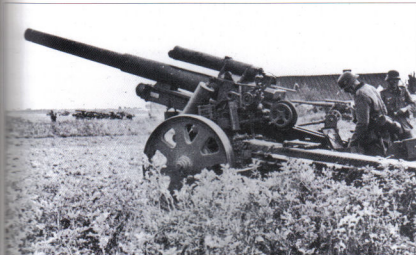
The backbone of German divisional artillery was the 150mm sFH 18, a modern weapon usually towed by a semi-tracked prime mover such as the SdKfz 7. (NARA)
